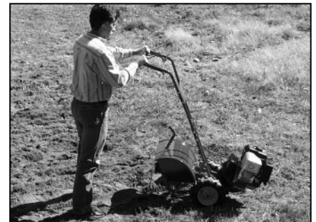
Fig. 4-3: To begin turn, lift handlebars until tines are out of ground and unit is balanced.
